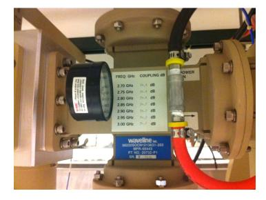
Loss from Transmitter Coupler 3DC1 is found here:
