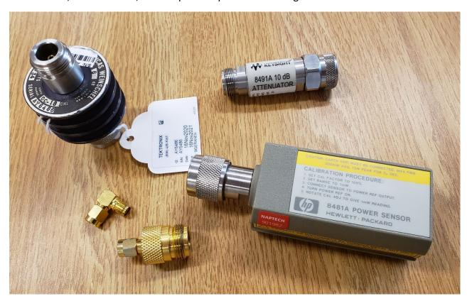
Attenuator, fixed, medium-power, 6 dB (Weinschel 23-6-34 or equivalent), Attenuator, fixed, low-power, 10 dB (HP8491A or equivalent), Power Sensor HP8481A or equivalent, (F) N-Type to (M) SMA adapter, SMA 90° adapter
